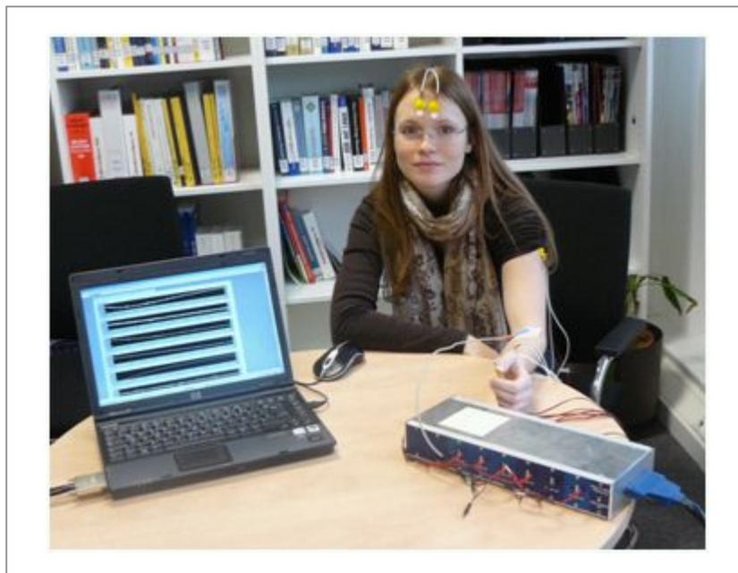
Figure 3.1 – Setup of first sensor sub-study
