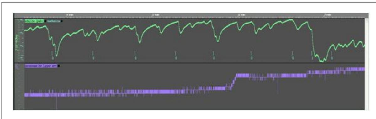
Figure 3.5 – Comparison of EDA recording at the palm and sensewear device at upper arm
